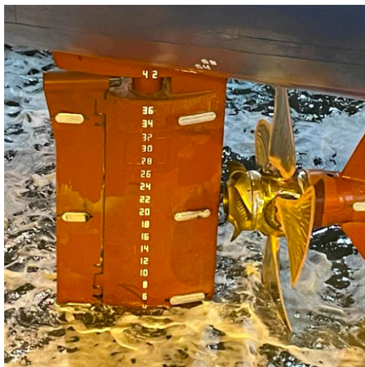
Leme do Navio Lagoa com pintura à base de silicone, Estaleiro Navalrocha, Janeiro 2023. Lagoa Vessel's Rudder painted with silicone painting, Navalrocha shipyard, January 2023.
